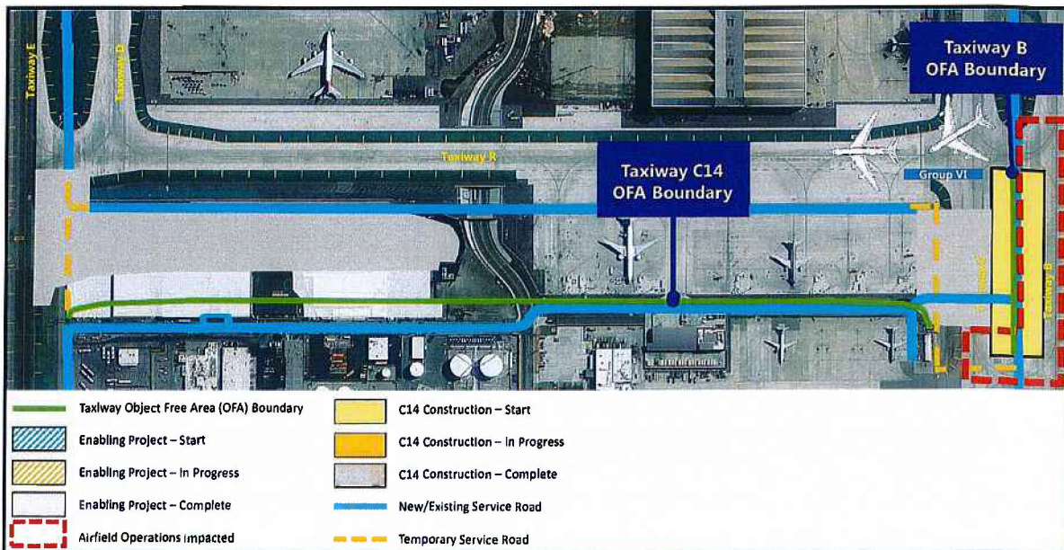
Figure 12 - Taxiway C14 Construction (Taxiway B)
